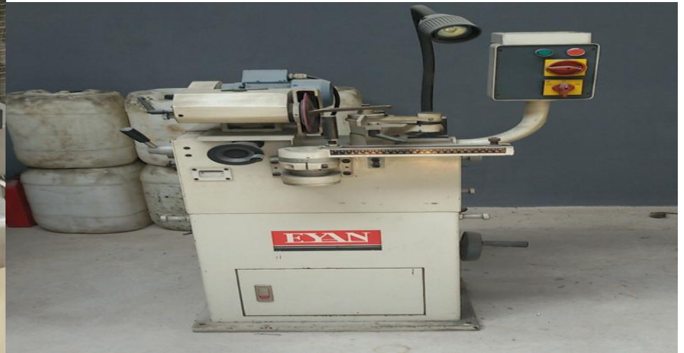
Mesin Re- Grinding Saw Blade
