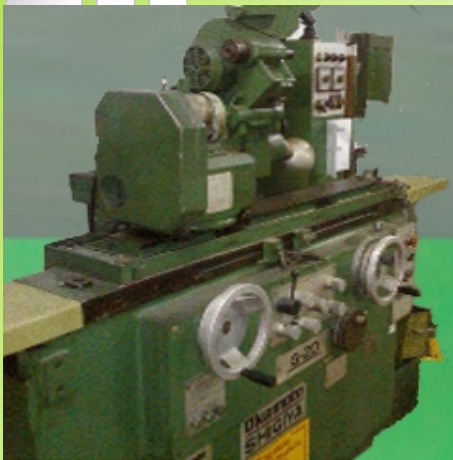
Cylindrical Grinding M/c, Okamoto Shigiya, GU-20-50 Ø 200 X 500
