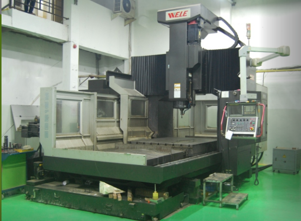
Mill CNC M/C, 5 Faces WELE- SB216M ( Double Coloumn) Table 2000x1600 x 800
