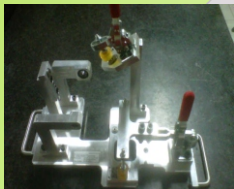
Jig Spot Welding
