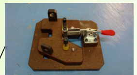
Jig Spot Welding
