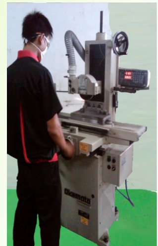
Precision Grinding M/c, Okamoto, ACC350ST #350 x 150 x 400
