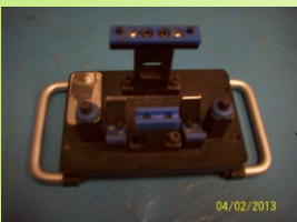
Jig Spot Welding
