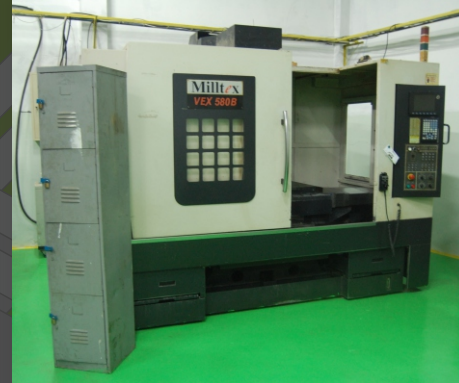
Mill CNC M/C Milltex, VBE-580B #1100 x 580 x 500
