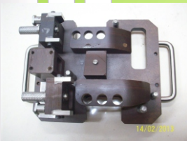
Jig Spot Welding
